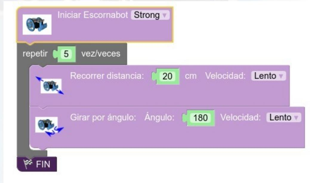
The image shows a Scratch script for a robot. It starts with a 'Start Robot' block set to 'Strong'. This is followed by a 'Repeat' loop block set to '5' times. Inside the loop, there are two blocks: 'Move distance' set to '20 cm' and 'Slow' velocity, and 'Turn by angle' set to '180' degrees and 'Slow' velocity. The script ends with a 'FIN' block.
